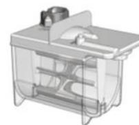
Tests can be performed on liquids, macerated solids or swabbed samples. In the event of a positive result (microbial contamination), Speedy Breedy alerts the operator and corrective action such as decontamination and sterilisation procedures can commence immediately.
